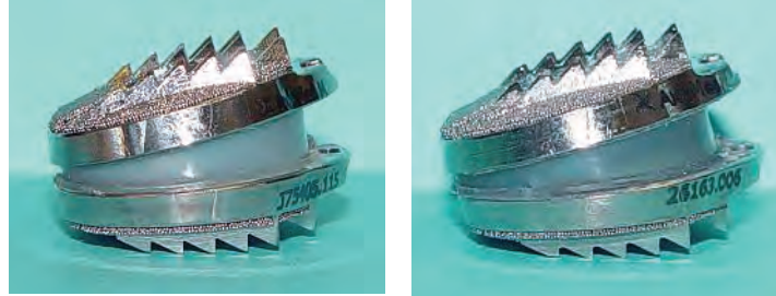
FIGURE 5: PHOTO OF UNTESTED FLD (LEFT) COMPARED TO FLD AFTER 10 MILLION CYCLES AT A COMPRESSIVE SHEAR LOAD OF 1,200 N. (ETC TECHNICAL REPORT 167-299201-27)
